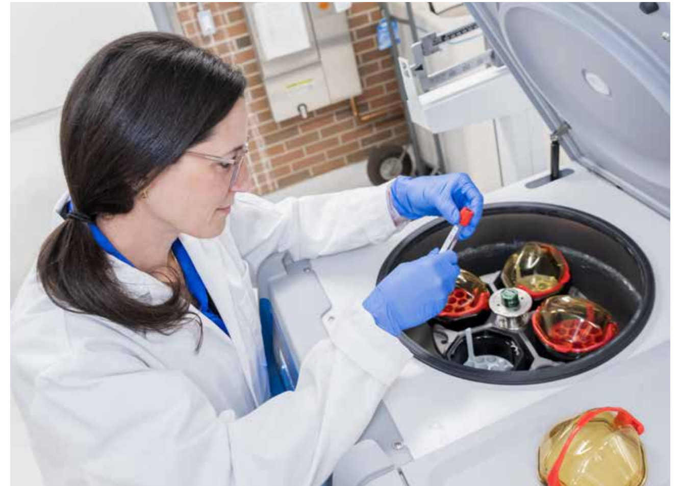
Josse puts a sample of a participant's blood into a centrifuge to collect the serum/plasma for analysis
